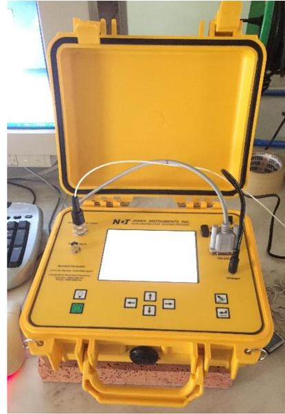
Fig.2-4-1: Resonant frequency tester (E-Meter Mk II)
