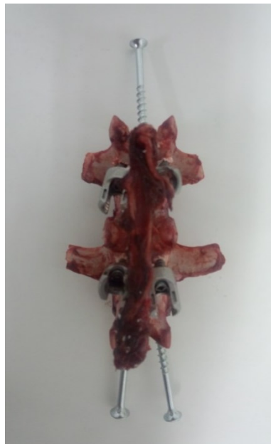
Fig.3.4 Specimen after screw insertion to vertebral body
