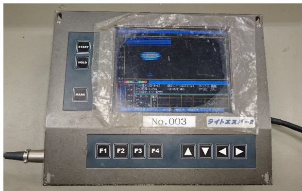
Fig. 2.2 Ground penetrating radar processing unit
