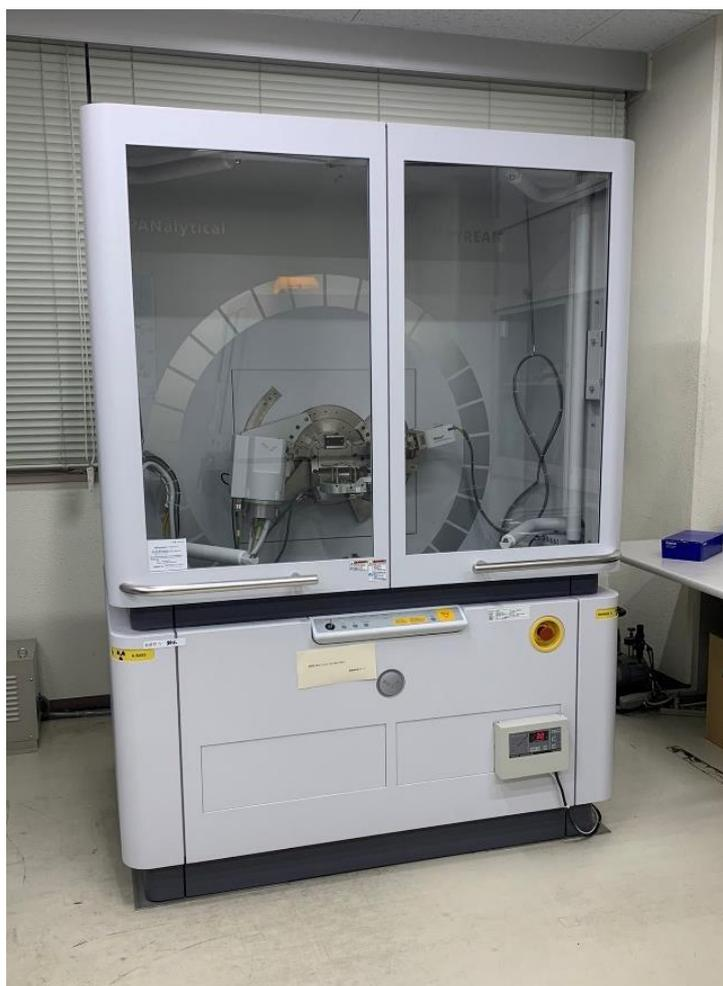
Fig. 3-3 X-ray diffractometer Empyrean.
