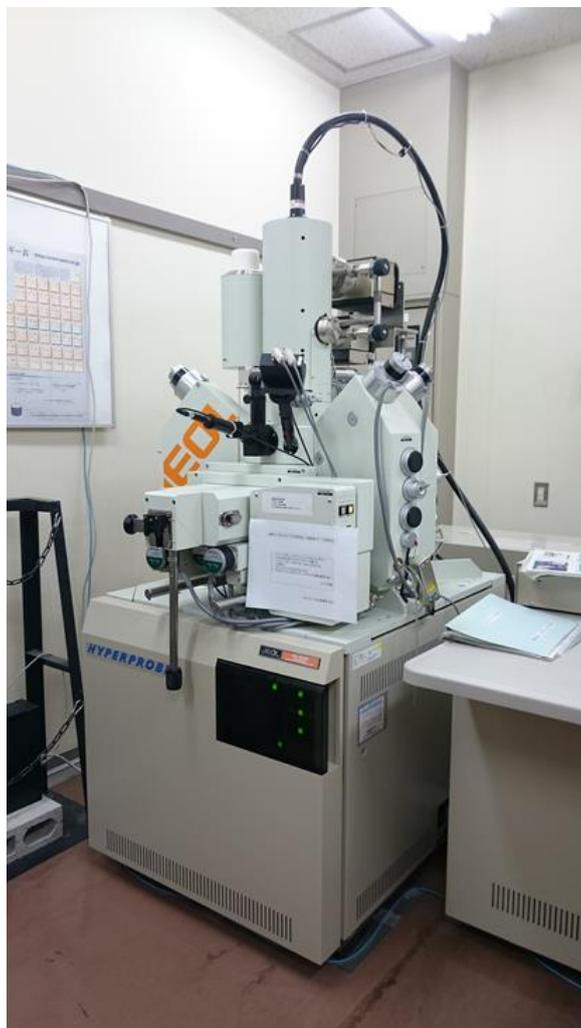
Fig. 3-2 Electron Probe Microanalyzer JXA-8530F.
