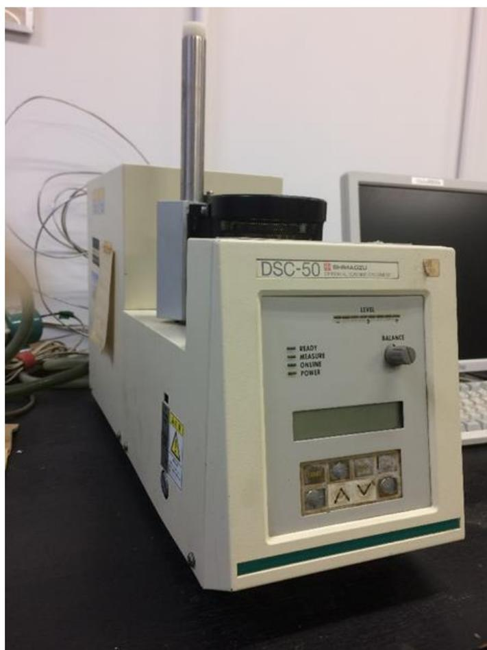
Fig. 3-5 Differential scanning calorimetry DSC-50.
