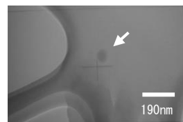
Fig. 3 contamination on old mesh
