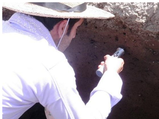
Photo 3.6 Soil hardness measurement by Yamanaka hardness meter
