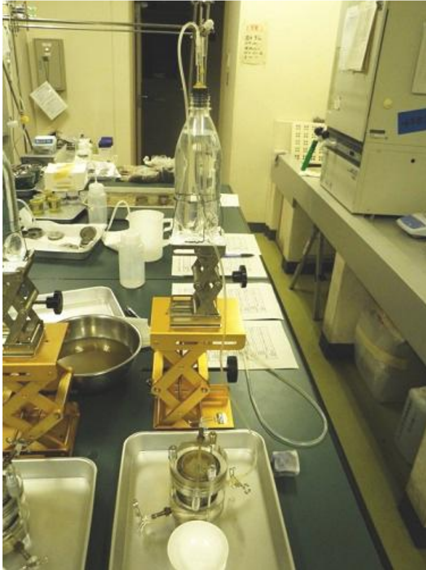
Photo 3.18 Constant head hydraulic conductivity system device and operation
