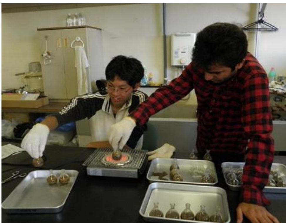
Photo 3.8 Heating the samples for air removal
