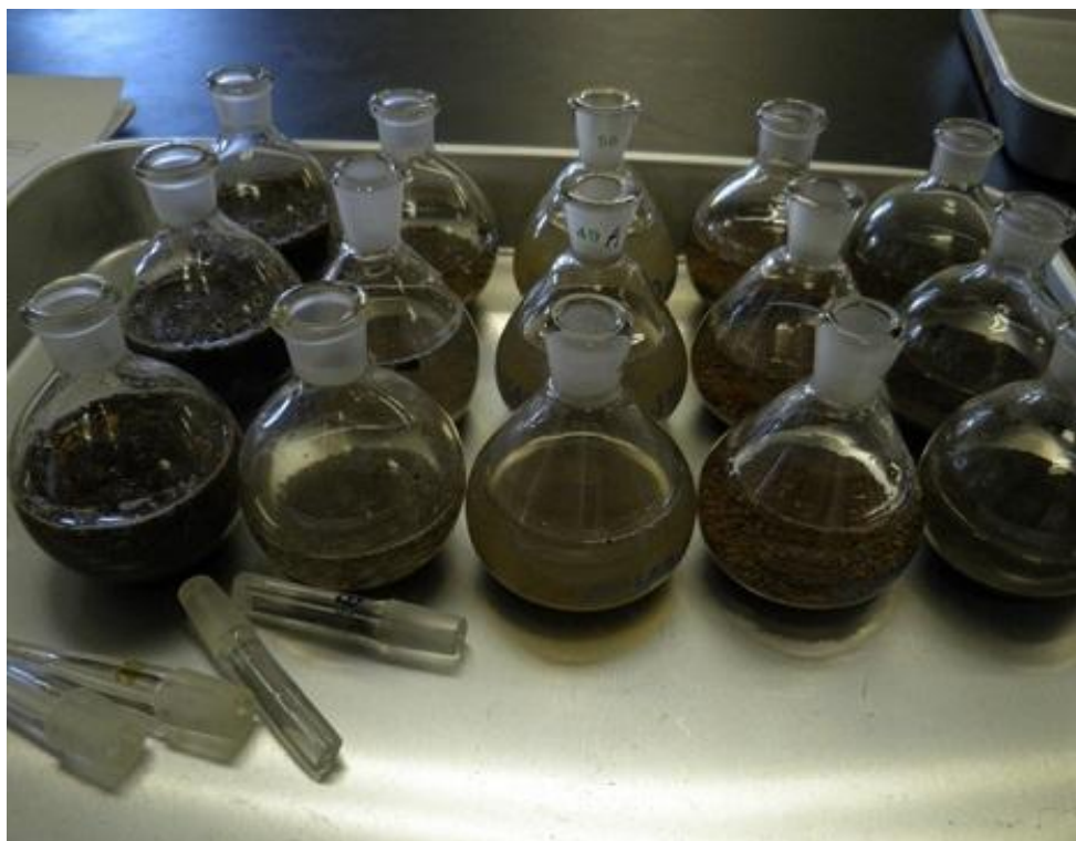
Photo 3.7 Samples placed in pycnometer
