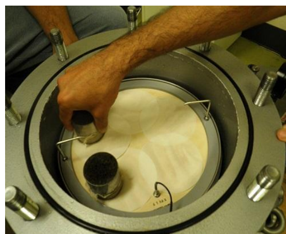
Photo 3.22 Placing samples on the ceramic plate inside pressure plate apparatus
