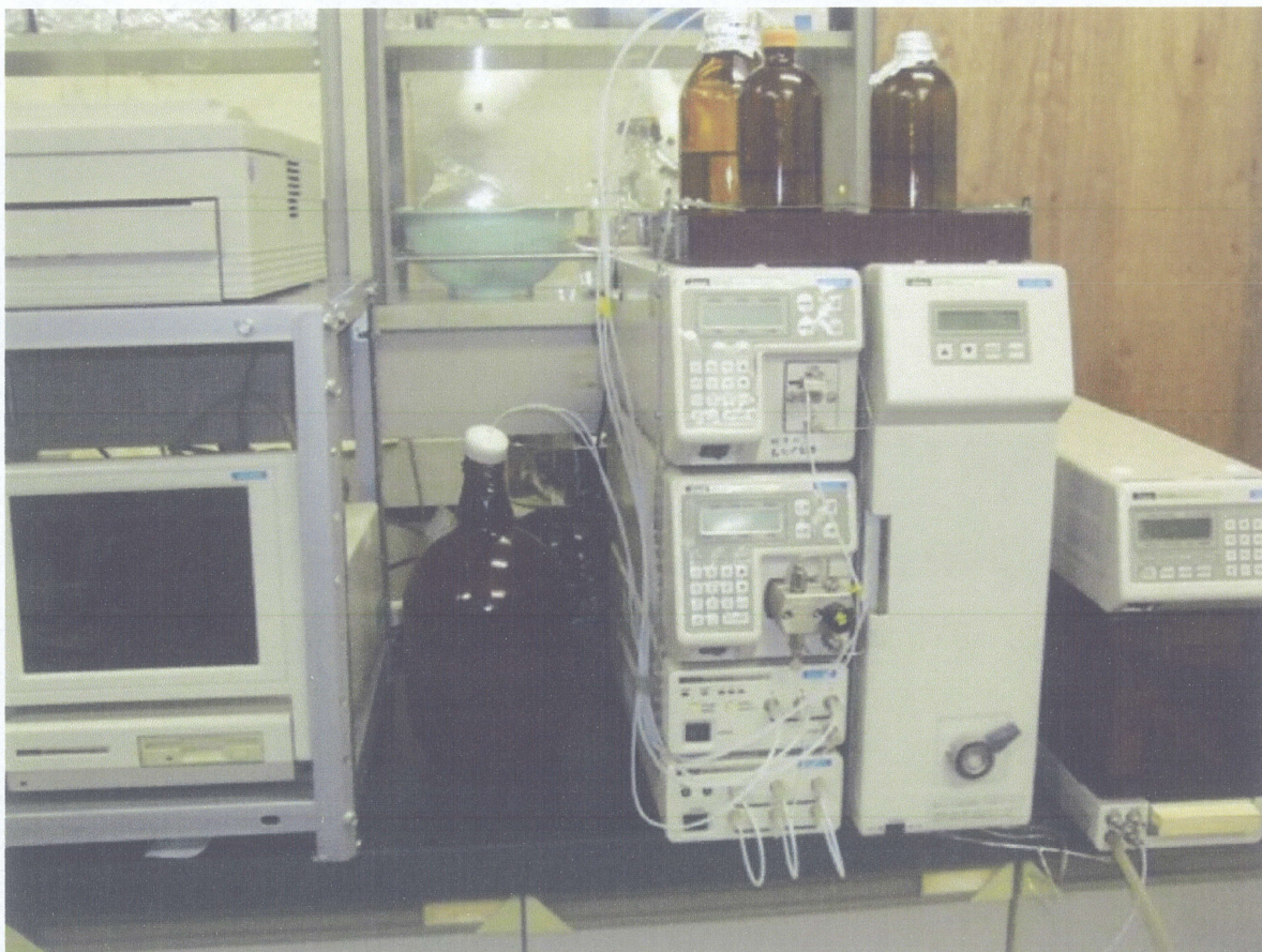
Fig. 5 The HPLC system for the analysis of ATP-related compounds.
