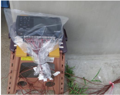
Photo 3.8 Data logger in outside irradiation test
