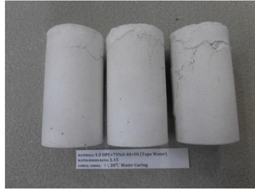
Materials: 1:2 OPC+75%S-40+OS (Tape Water) Curing: 20°C Water Curing
