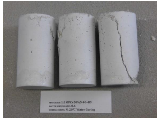
Materials: 1:3 OPC+50%S-40+RS Curing: 20°C Water Curing
