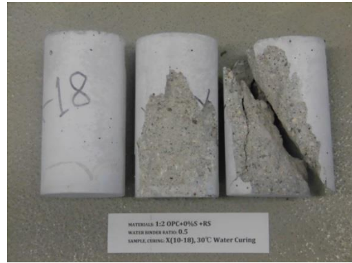
Materials: 1:2 OPC+0%S +RS Curing: 30°C Water Curing
