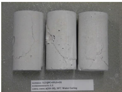
Materials: 1:2 QPC+0%S+OS Curing: 30°C Water Curing
