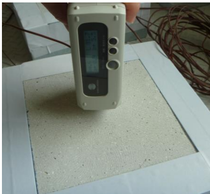
Photo 3.5 Brightness test with digital color reader
