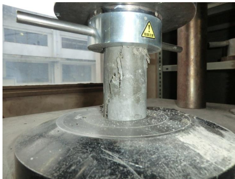
Photo 2.12 Photographic view of the compressive strength test by universal testing machine
