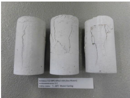
Materials: 1:2 OPC+0%S +OS (Sea Water) Curing: 20°C Water Curing
