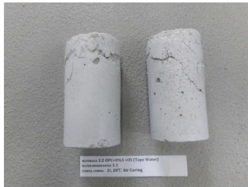
Materials: 1:2 OPC+0%S +OS (Tape Water) Curing: 20°C Air Curing
