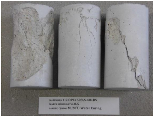
Materials: 1:2 OPC+50%S-40+RS Curing: 20°C Water Curing
