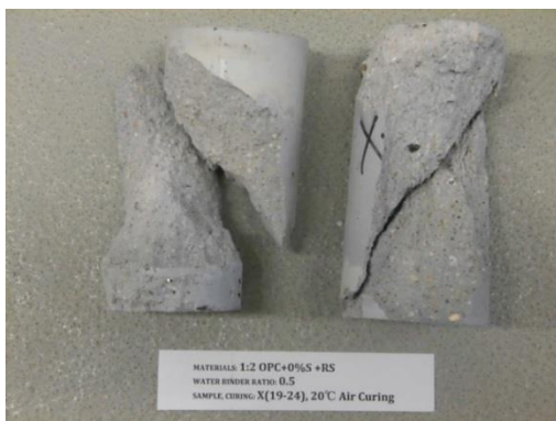
Materials: 1:2 OPC+0%S +RS Curing: 20°C Air Curing
