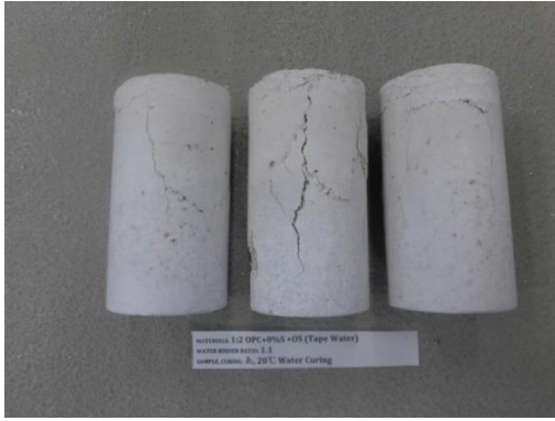
Materials: 1:2 OPC+0%S +OS (Tape Water) Curing: 20°C Water Curing
