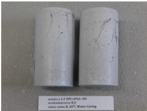
Materials: 1:2 OPC+0%S+RS Curing: 20°C Water Curing
