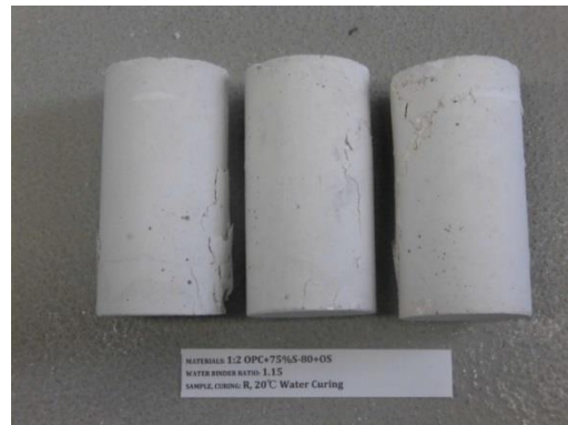
Materials: 1:2 OPC+75%S-80+OS Curing: 20°C Water Curing
