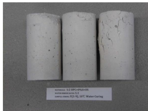
Materials: 1:2 OPC+0%S+OS Curing: 10°C Water Curing
