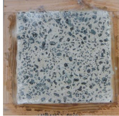
Photo 3.4 Mortar filled pavement
