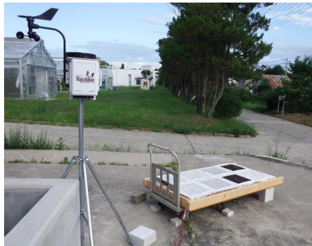
Photo 3.10 Light irradiation test in open and natural condition
