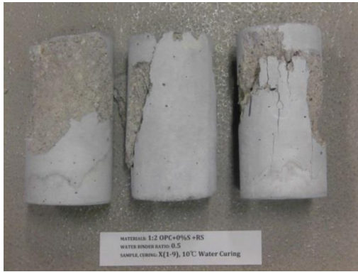
Materials: 1:2 OPC+0%S +RS Curing: 10°C Water Curing
