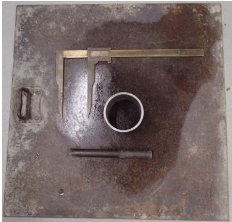
Photo 2.9 Flow measuring instrument
