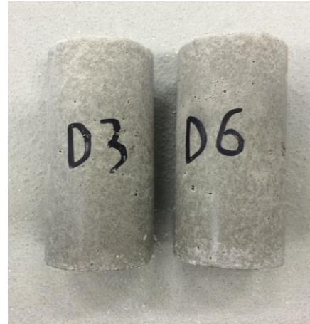
Photo 2.11 Compressive strength test sample
