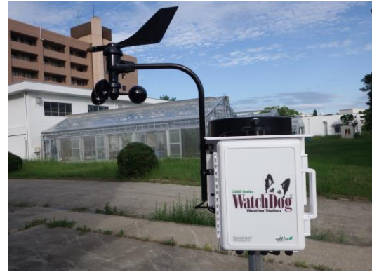
Photo 3.9 Weather station for measuring weather data
