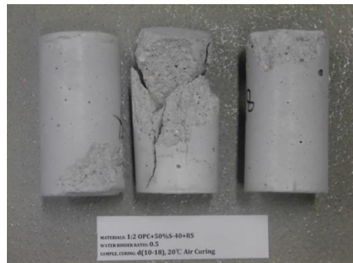
Materials: 1:2 OPC+50%S-40+RS Curing: 20°C Air Curing
