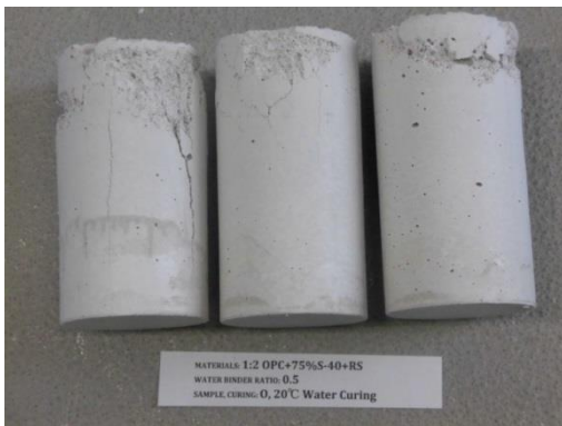
Materials: 1:2 OPC+75%S-40+RS Curing: 20°C Water Curing
