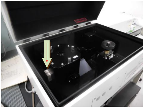
Photo 3.11 Sample inside the spectrometric radiation reflection measuring machine
