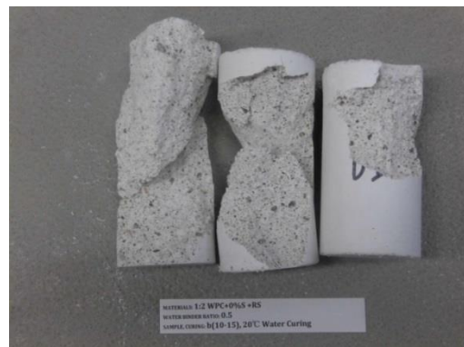
Materials: 1:2 WPC+0%S+RS Curing: 20°C Water Curing
