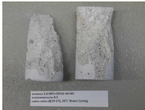
Materials: 1:2 OPC+50%S-40+RS Curing: 30°C Water Curing
