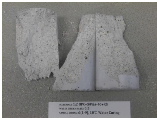
Materials: 1:2 OPC+50%S-40+RS Curing: 10°C Water Curing
