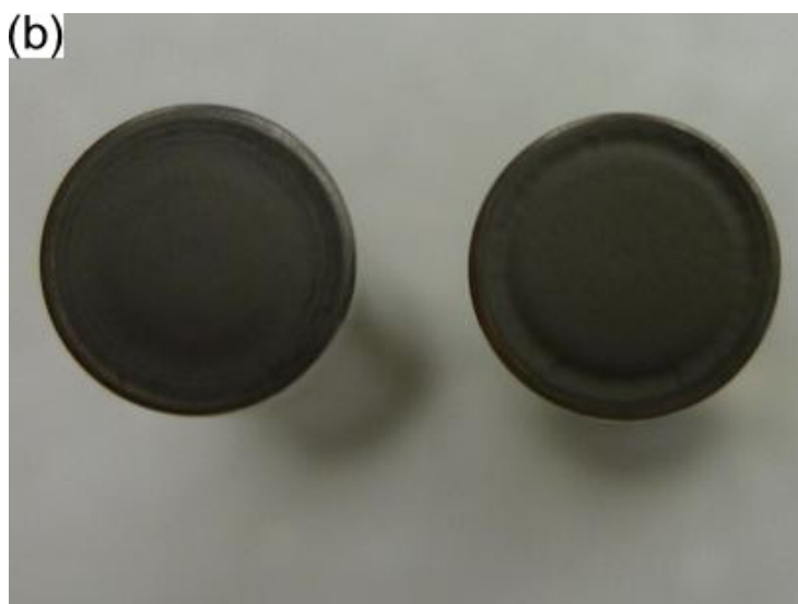
Fig. 6. (a) Black sediment at the bottom of a sample sonicated by a probe-type sonicator at 20 W, 80% pulse mode, for 30 min after 2 hours on standing and (b) the tip surface of unused probe (left) and abraded probe (right).
