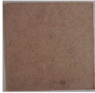
biomass board LF-2: 4\text{mm} < \text{fiber length} \leq 5.6\text{mm} , applied pressure was 3.5\text{MPa}
