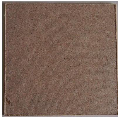
a. biomass board A (heating temperature was 110°C)
