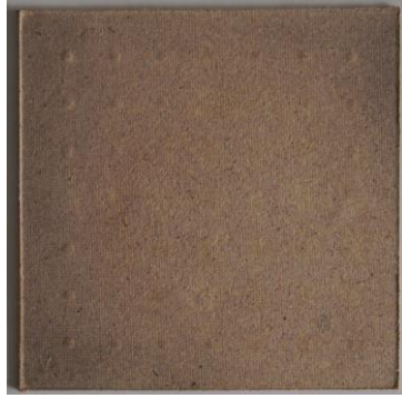
biomass board SF-3: 0\text{mm} < \text{fiber length} \leq 2.0\text{mm} , applied pressure was 5.0\text{MPa}
