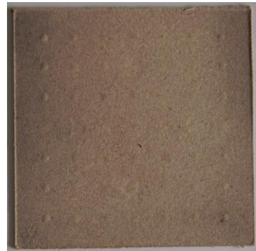
biomass board SF-5: 0\text{mm} < \text{fiber length} \leq 2.0\text{mm} , applied pressure was 8.0\text{MPa}
