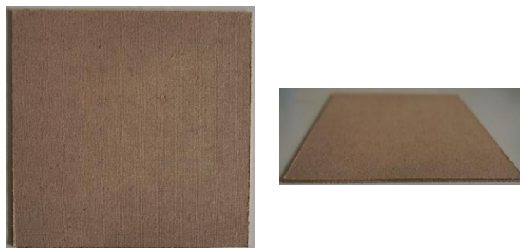
biomass board SF-2: 0\text{mm} < \text{fiber length} \leq 2.0\text{mm} , applied pressure was 3.5\text{MPa}
