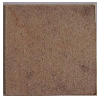
biomass board LF-5: 4\text{mm} < \text{fiber length} \leq 5.6\text{mm} , applied pressure was 8.0\text{MPa}
