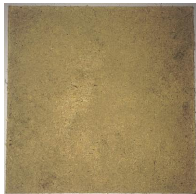
b. biomass board B (heating temperature was 130°C)
