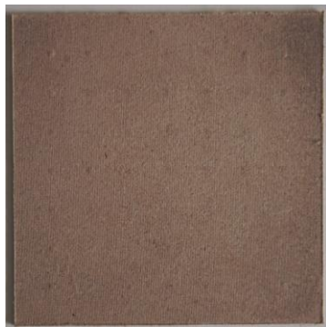
biomass board SF-4: 0\text{mm} < \text{fiber length} \leq 2.0\text{mm} , applied pressure was 6.5\text{MPa}
