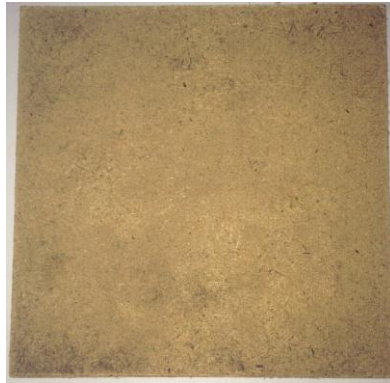
d. biomass board D (heating temperature was 170°C)
