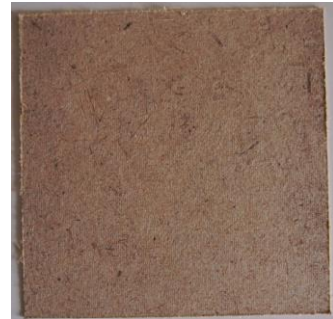
biomass board LF-4: 4\text{mm} < \text{fiber length} \leq 5.6\text{mm} , applied pressure was 6.5\text{MPa}
