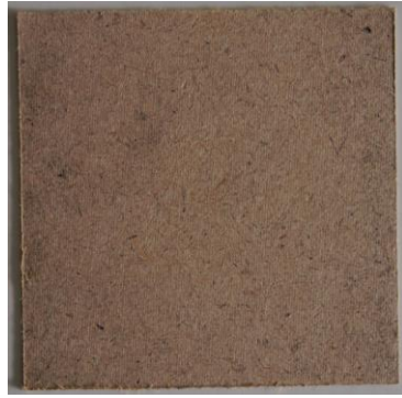
biomass board MF-4: 2\text{mm} < \text{fiber length} \leq 4.0\text{mm} , applied pressure was 6.5\text{MPa}
