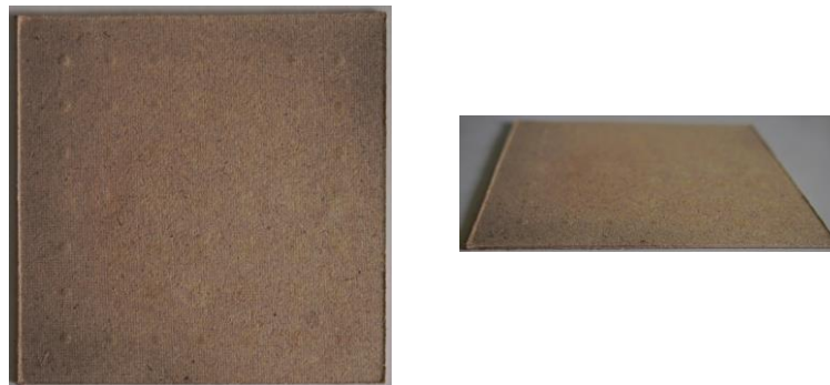
biomass board SF-1: 0\text{mm} < \text{fiber length} \leq 2.0\text{mm} , applied pressure was 2.0\text{MPa}
