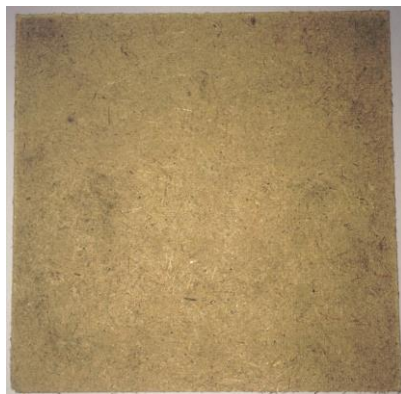
e. biomass board E (heating temperature was 190°C)
