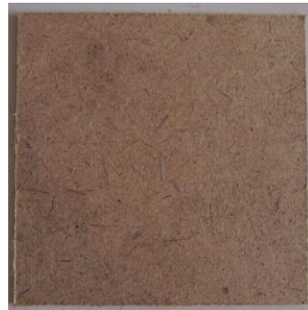
biomass board LF-3: 4\text{mm} < \text{fiber length} \leq 5.6\text{mm} , applied pressure was 5.0\text{MPa}
