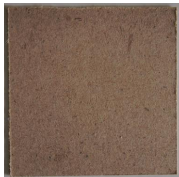
biomass board MF-3: 2\text{mm} < \text{fiber length} \leq 4.0\text{mm} , applied pressure was 5.0\text{MPa}
