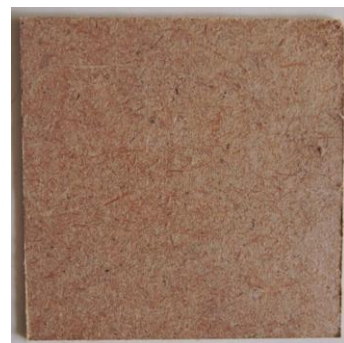
biomass board LF-1: 4\text{mm} < \text{fiber length} \leq 5.6\text{mm} , applied pressure was 2.0\text{MPa}
