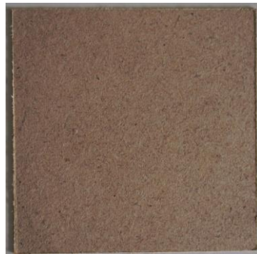
biomass board MF-2: 2\text{mm} < \text{fiber length} \leq 4.0\text{mm} , applied pressure was 3.5\text{MPa}
