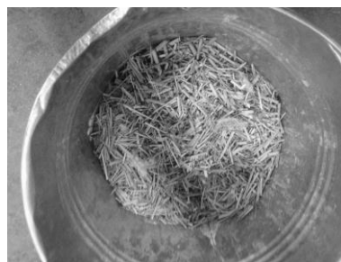
Fig.2- 7 The chips were cut by an ordinary cutter
