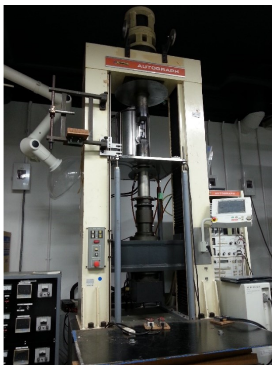
Fig. 3-3 Multi loading test machine with electric furnace (Autograph AG-10TC-IR) .
