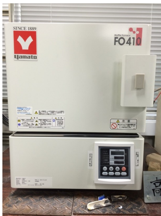
Fig.3-2 Muffle furnace FO410 to anneal specimens.
