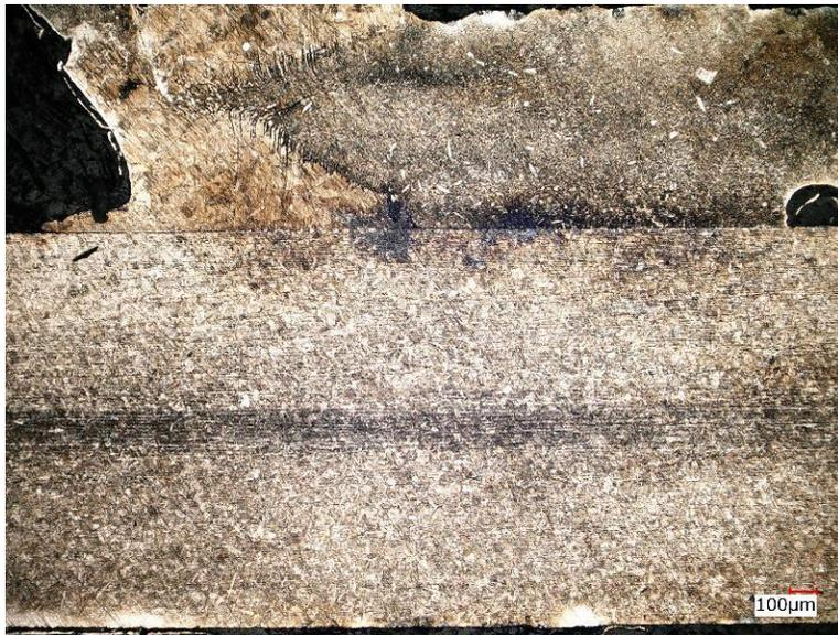
Fig.4-1 Section observation result after welding of 6cycle,8.0kA,1kN using R type
