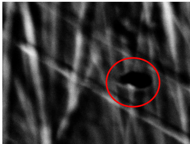
Fig.4-21 Black particles inside molten metal of SWRM10.
