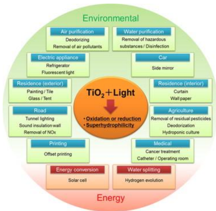
Figure 1.6. Applications of \text{TiO}_2 photocatalysis (Reproduced from [189] with permission from Elsevier).
