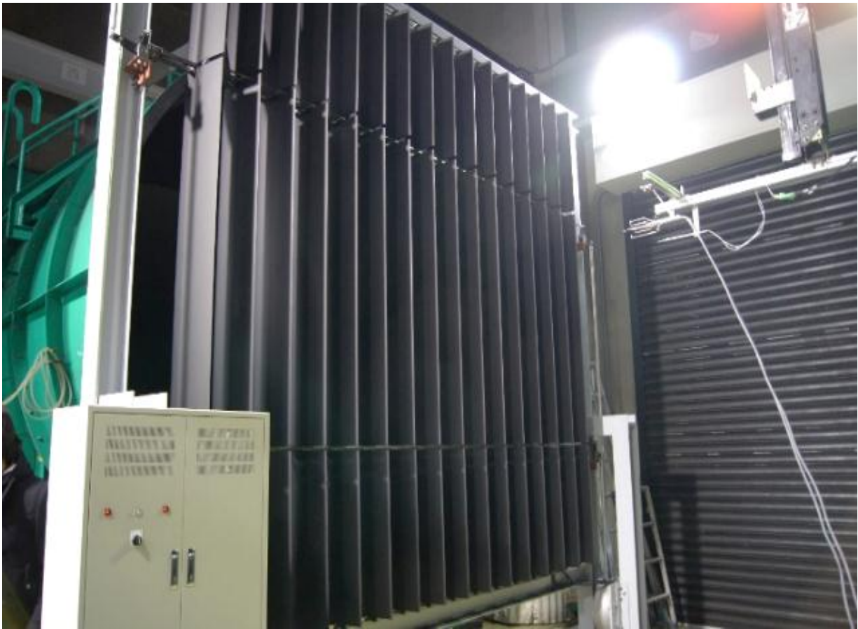
Fig. 5.3 Wind direction change equipment in wind tunnel
