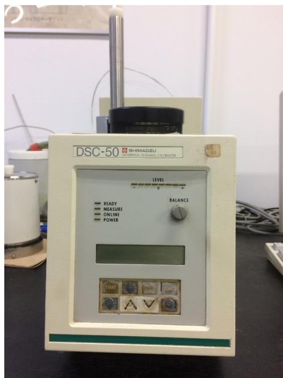
Fig.3-3 Differential scanning calorimetry DSC-50.
