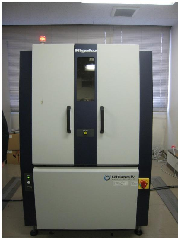
Fig.3-5 X-ray diffractometer Ultima IV.
