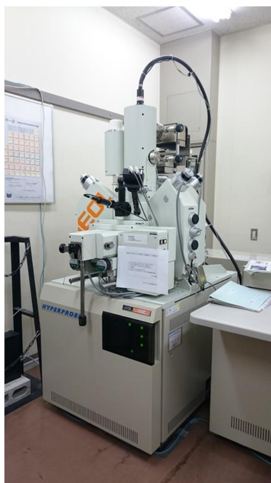
Fig.3-2 Electron Probe Microanalyzer JXA-8530F.
