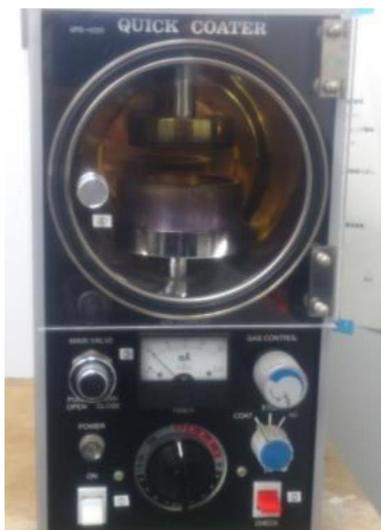
**Fig.4-7 Vacuum evaporation system**
