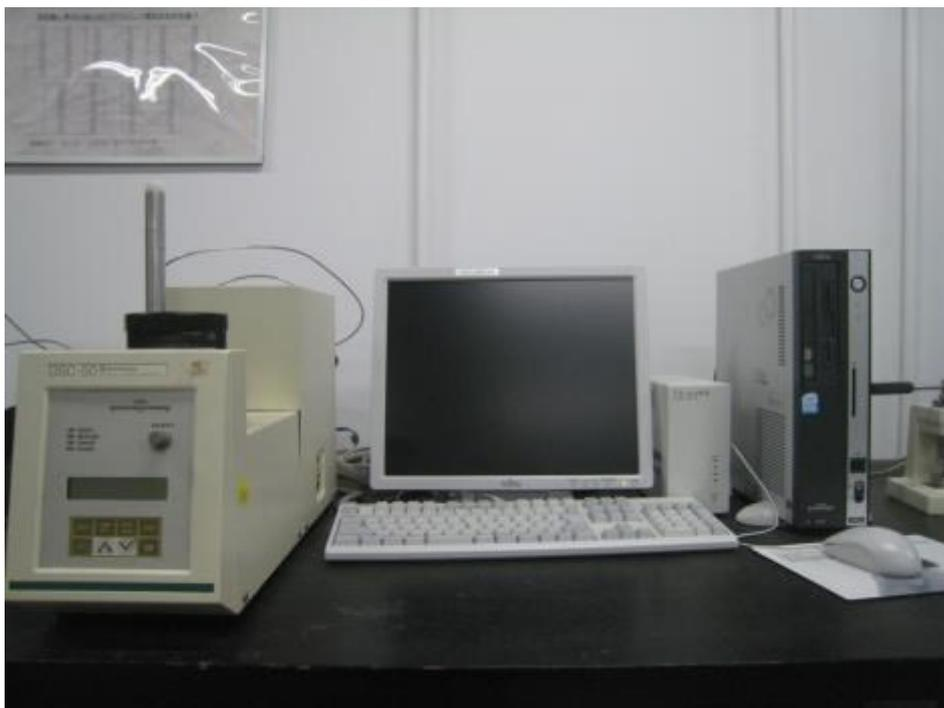
**Fig.4-2 Differential scanning calorimeter (DSC)**
