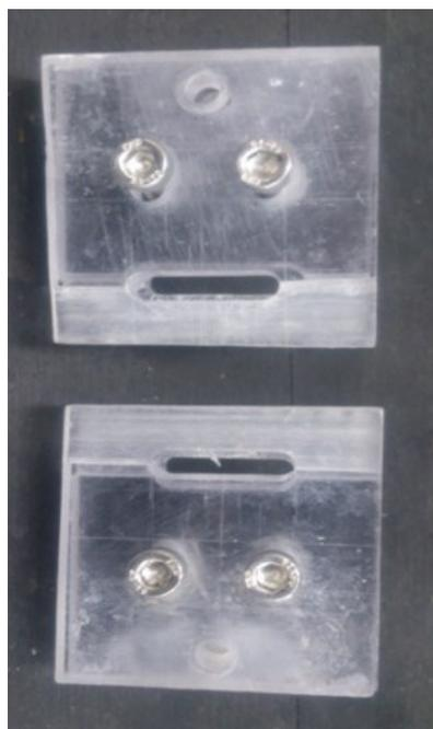
**Fig.4-4 Jig for tensile testing**
