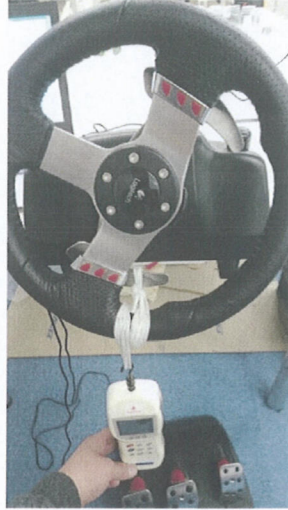
Fig. 4.5 Environment of experiment for measuring torque
