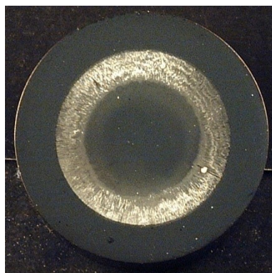
Fig.3.34 圧縮後工具表面 (Too-1, DLC-B, A1050-H, e_c=52\% )
