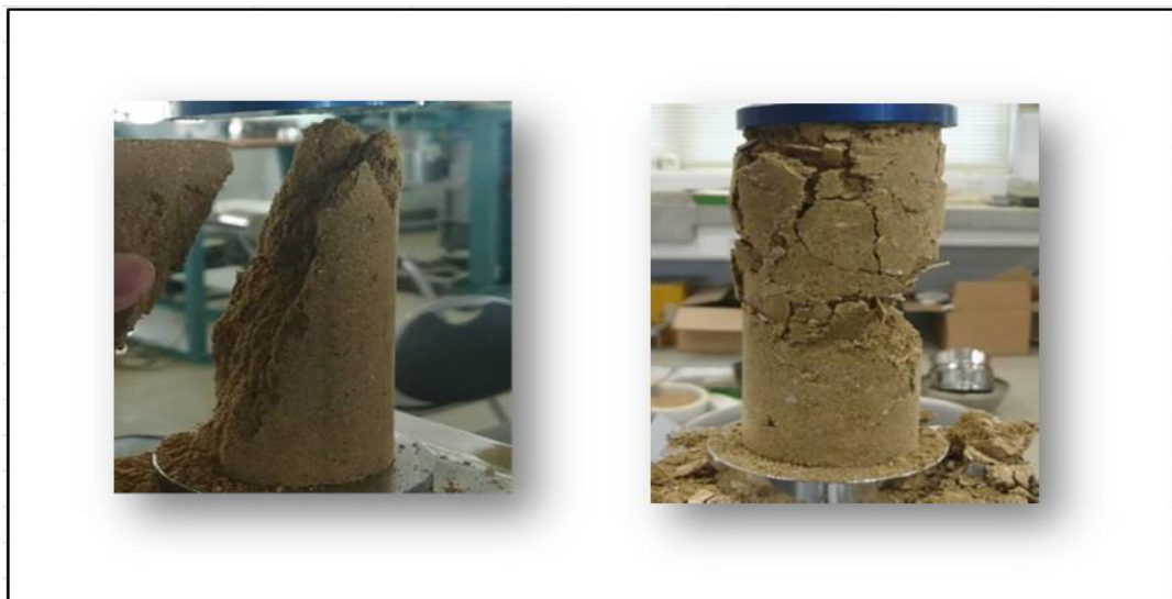
Figure 5. 25 Failure mode of control sample (left) and soil-shell husk-cement (right)
