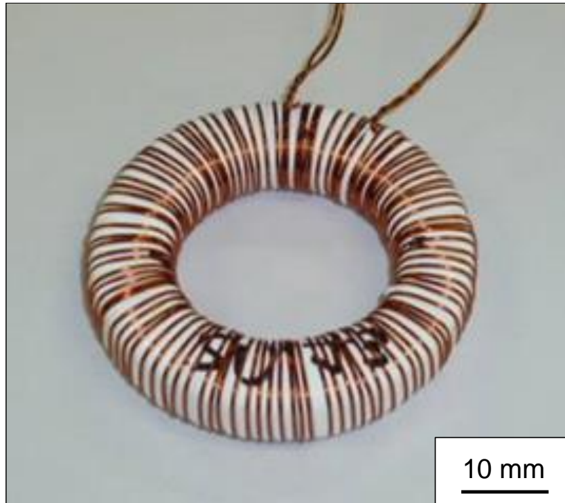
Fig. 4-2 Ring-shape specimen with solenoid coil used for the measurement of B - H curve.
