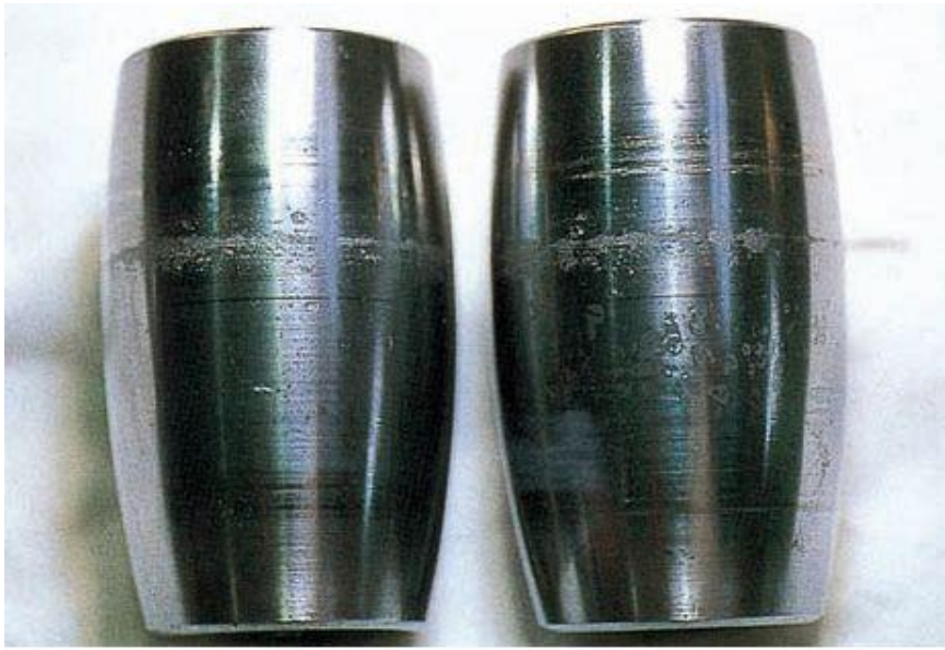
Fig. 1-9 Trace of peeling in the roller of a self-aligning roller bearing. 18)
