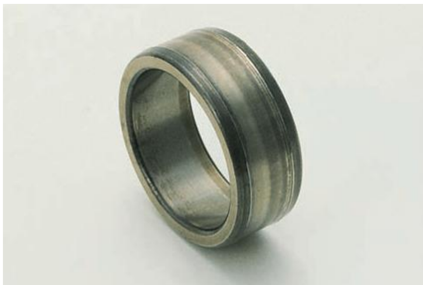
Fig. 1-11 Trace of wear in the inner raceway of a cylindrical roller bearing. 18)
