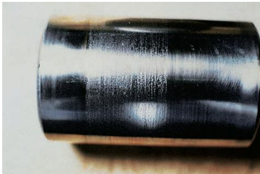
Fig. 1-10 Trace of smearing in the roller of a cylindrical roller bearings. 18)
