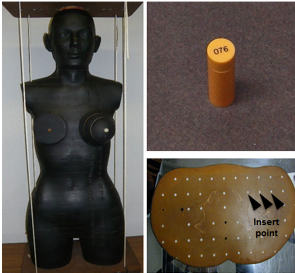
Fig. 2 Anthropomorphic phantom. Left panel shows the Rand Phantom. Right upper panel shows a radiophotoluminescence glass dosimeter. The glass dosimeters are inserted in the 37 position of an anthropomorphic Rando Phantom (Right lower panel)
