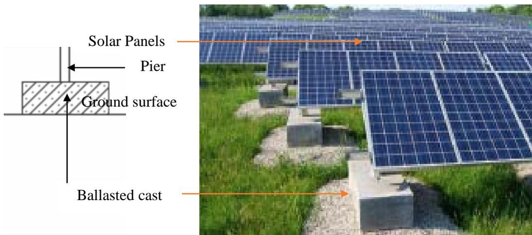
Figure 4: ballasted foundations set-up.
