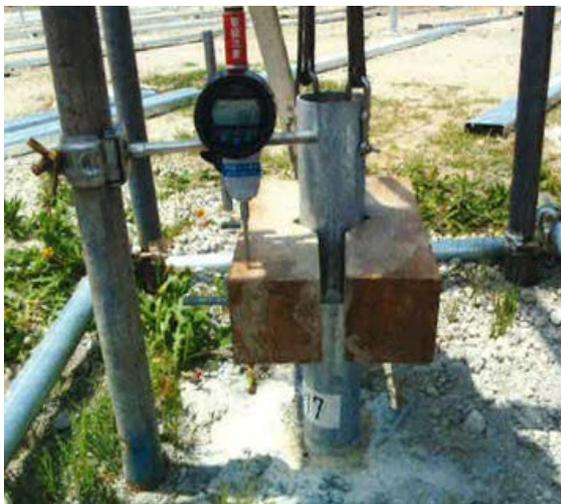
Figure 24 LVDT for vertical displacement
