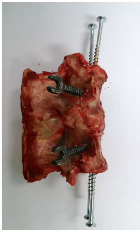
Fig.4.2 FSU with screw insertion to vertebral body
