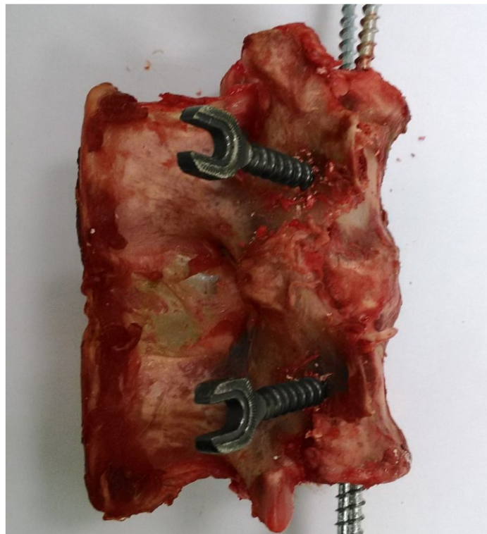
Fig.4.1 Specimen after pedicle screw insertion
