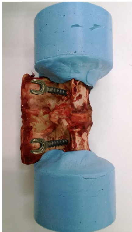
Fig.4.3 FSU with resin fixation
