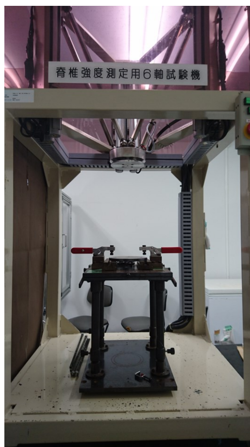
Fig.3.9 Six-axis material testing machine
