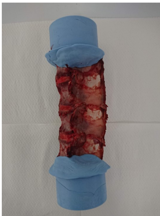
Fig.4.3 Specimen with resin fixation
