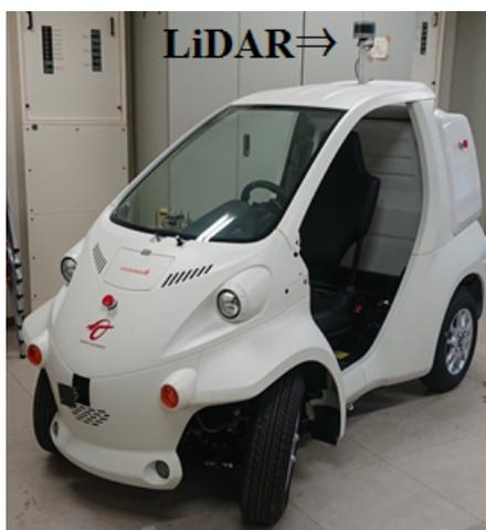
Fig. 3.1 COMS with LiDAR
