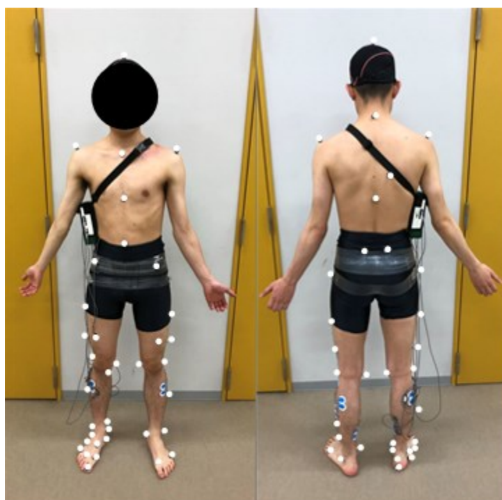
Fig.4.10 The location of reflecting markers and surface EMG
