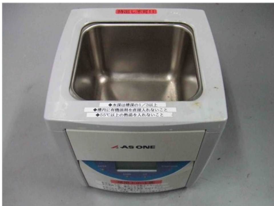
Fig.3-2 Ultrasonic cleaning process machine
