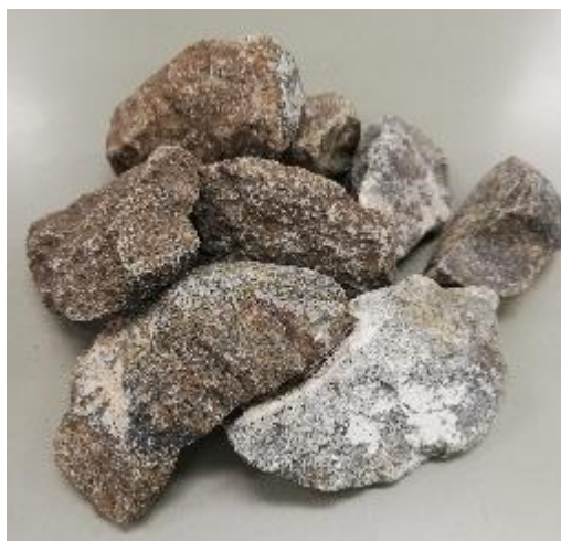
Fig.2.4 Crushed stone used in substations
