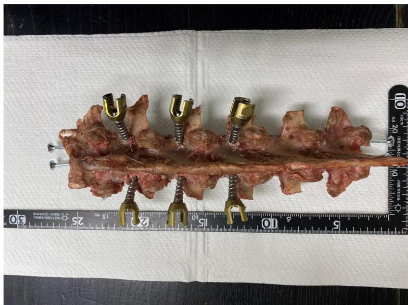
Fig. 4.1 Specimen after screw insertion to vertebral body
