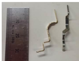
Fig.1.3 Example of connector terminals
