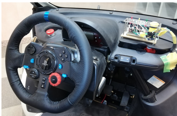
Fig. 5.2 Steering wheel G29 on the vehicle
