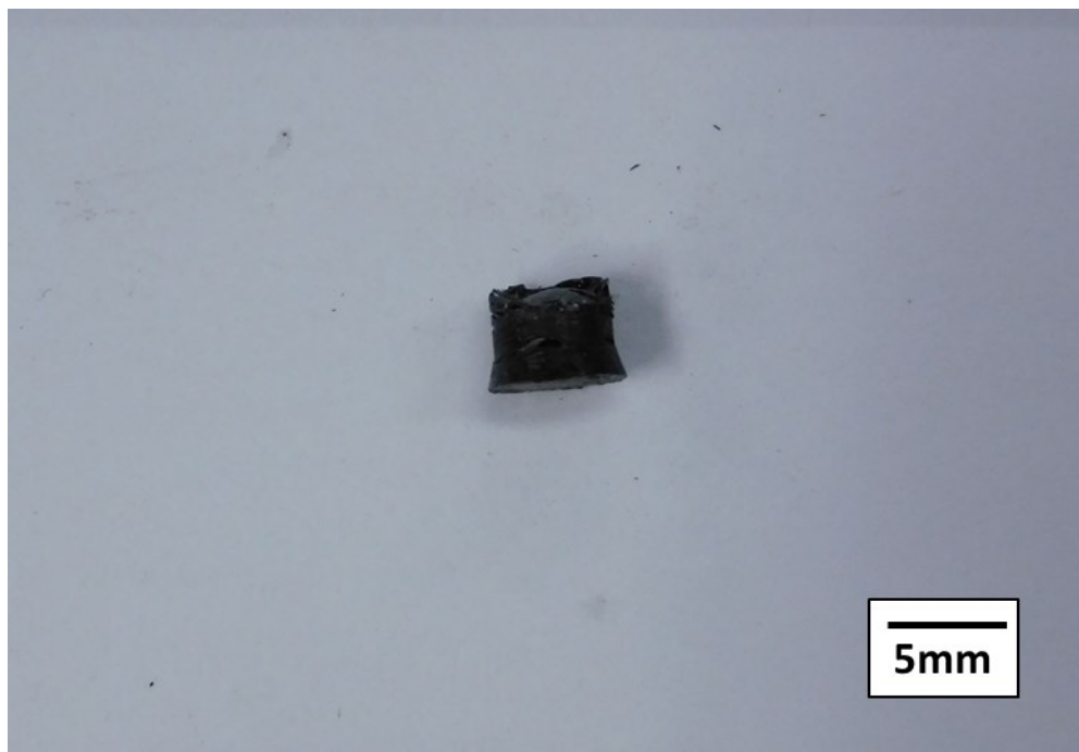
Fig. 3.6 Machining waste (CFRTP plate)
