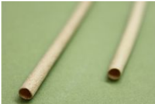
Fig. 2 Appearance of extruded pipe named “wood straws”.
