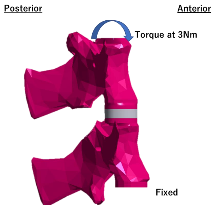
Fig. 3.10 Constraint and load conditions for an analysis simulating the spine pre flexion test
