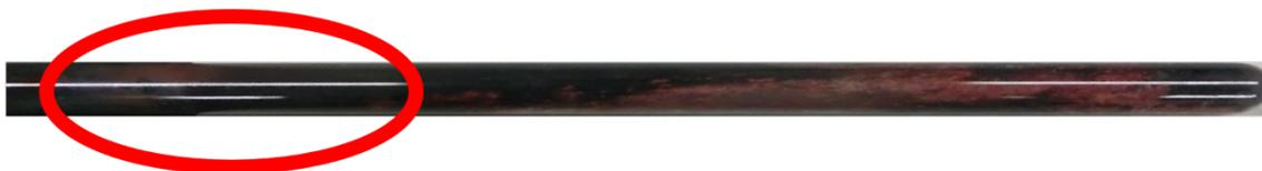
Figure 2-11 Quartz thin tube after Rapid Oxidation Reaction and collection position of product.
