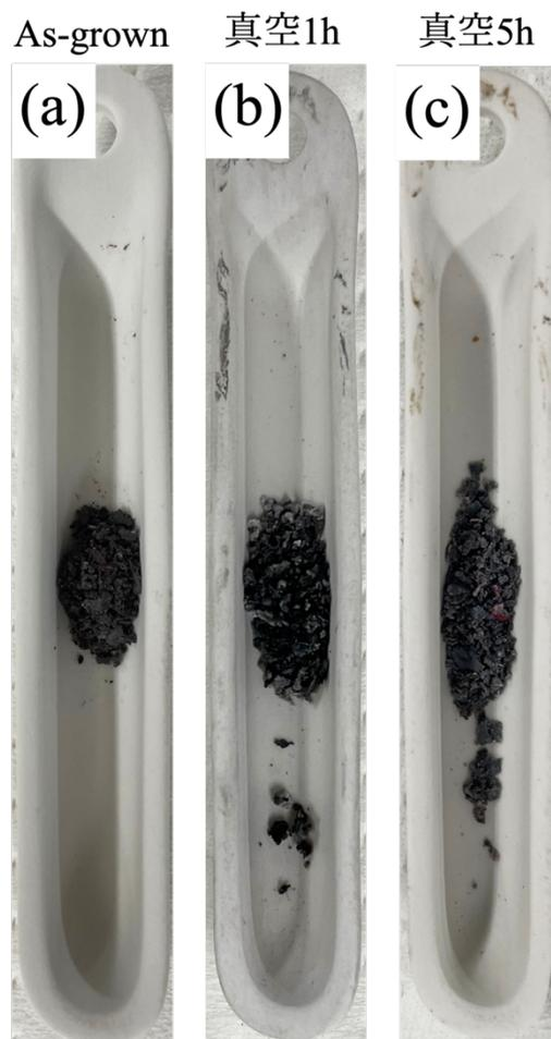
**Figure 3-17** Optical photographs of samples before and after vacuum heat treatment; (a) Before vacuum heat treatment, (b) After 1 hour vacuum heat treatment, (c) After 5 hours vacuum heat treatment.
