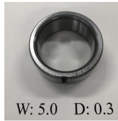
Fig.5.18 Inner ring faulty bearing
