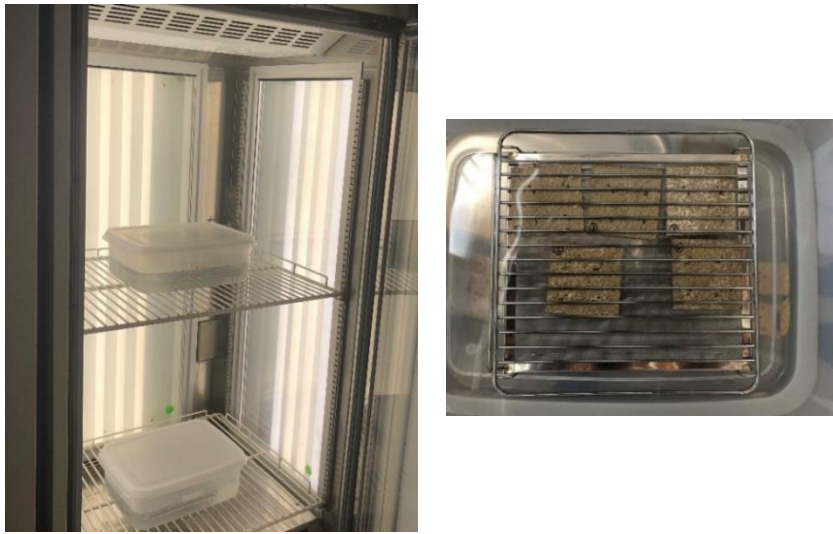
Fig.2-13 Incubator and specimens used in water absorption test
