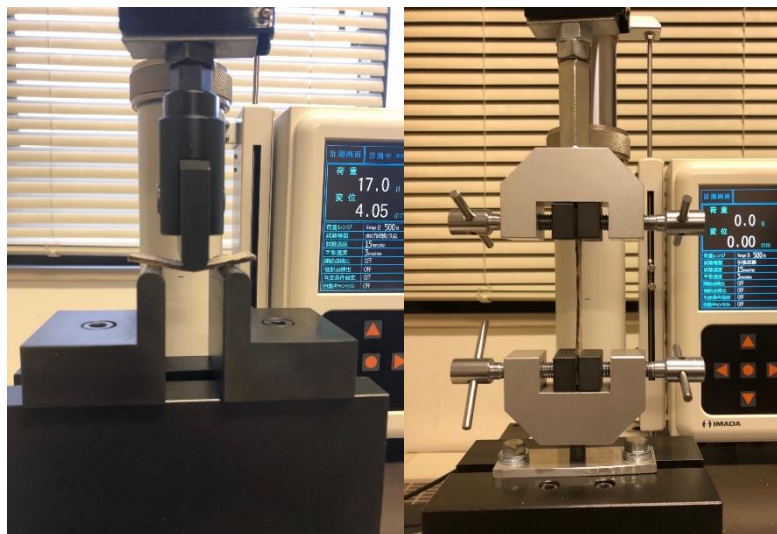
Fig.2-9 Three-point bending test and tensile test of bio-board.
