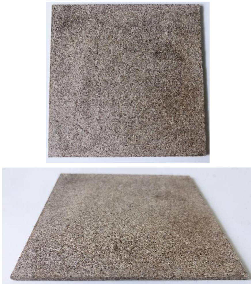
Fig.7-2 Surface and cross-section of produced hybrid bio-board
