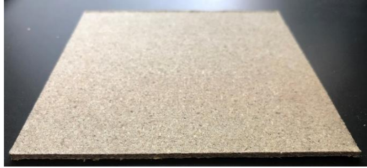
Fig.3-1 Produced bio-board at applied pressure of 5MPa.
