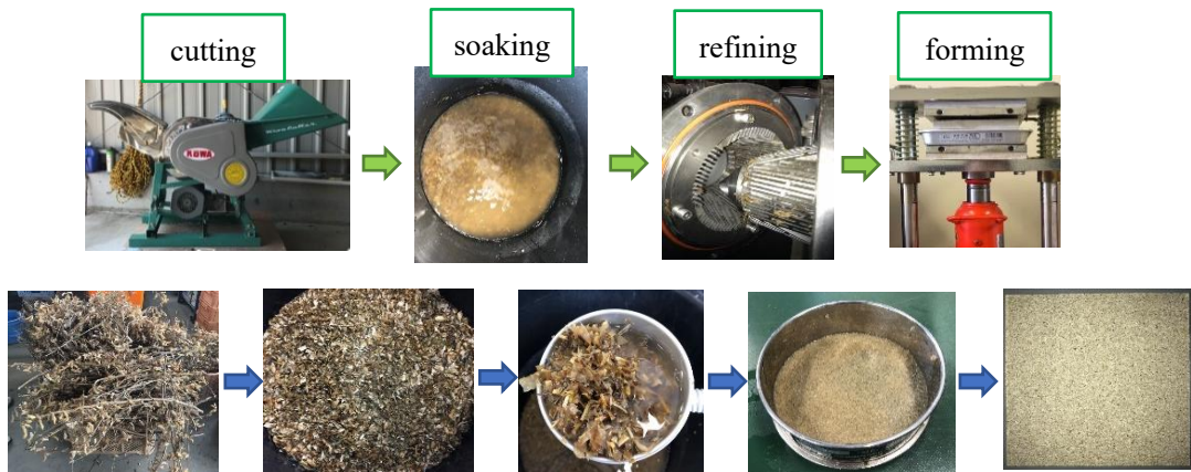
Fig.2-1 The making process of bio-board.
