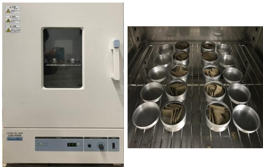
Fig.2-11 Dry oven and specimens for measuring the moisture content
