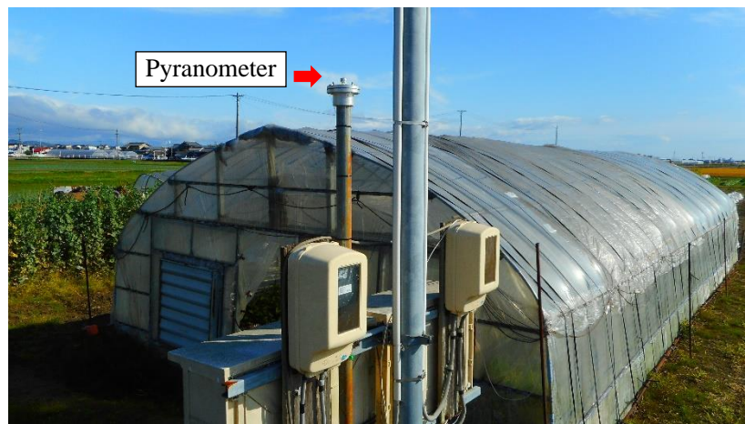
Figure 3-6 Measurement of relative humidity, solar radiation and air temperature inside the greenhouse
