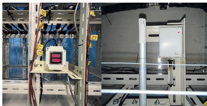
Figure 3-22 (b) Humidity sensor placed below a pipe (with and without monitor)
