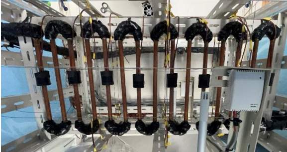
Figure 3-14 (b) Showing a serpentine copper pipe heat exchanger place on the stand (Top view)
