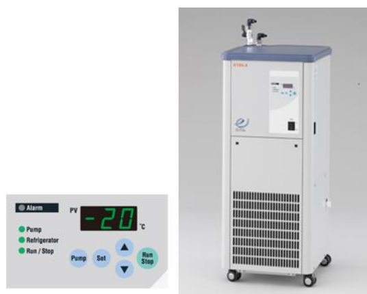
Figure 3-26 Photo of air-cooled chiller
