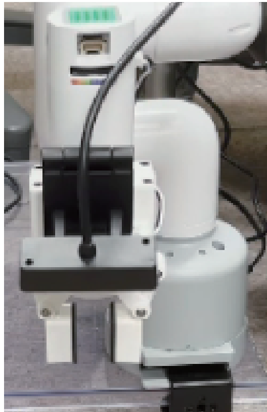
Fig. 4.12 Webcamera mounted on end effector
