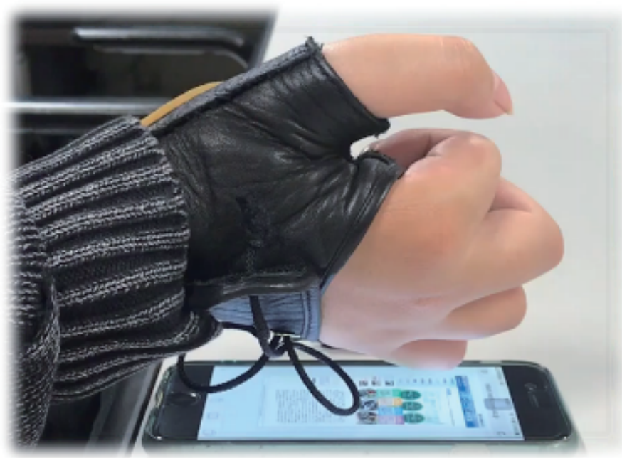
Fig. 4.15 Operation with the second joint of little finger
