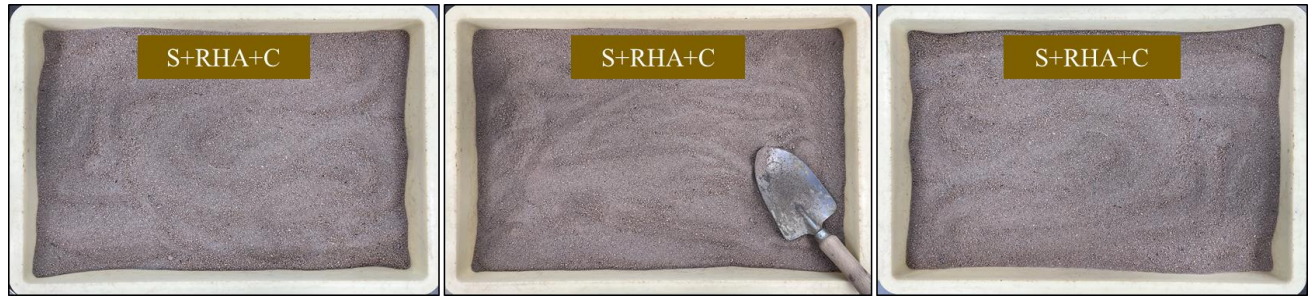
Figure 26 (a) Step 1: Dry mixing of Soil, RHA, and Cement in specified combinations.
