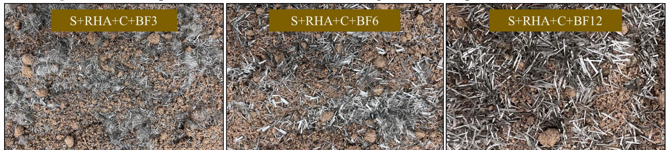
Figure 26 (c) Step 3: Addition of varied basalt fiber filament lengths in specified combinations.
