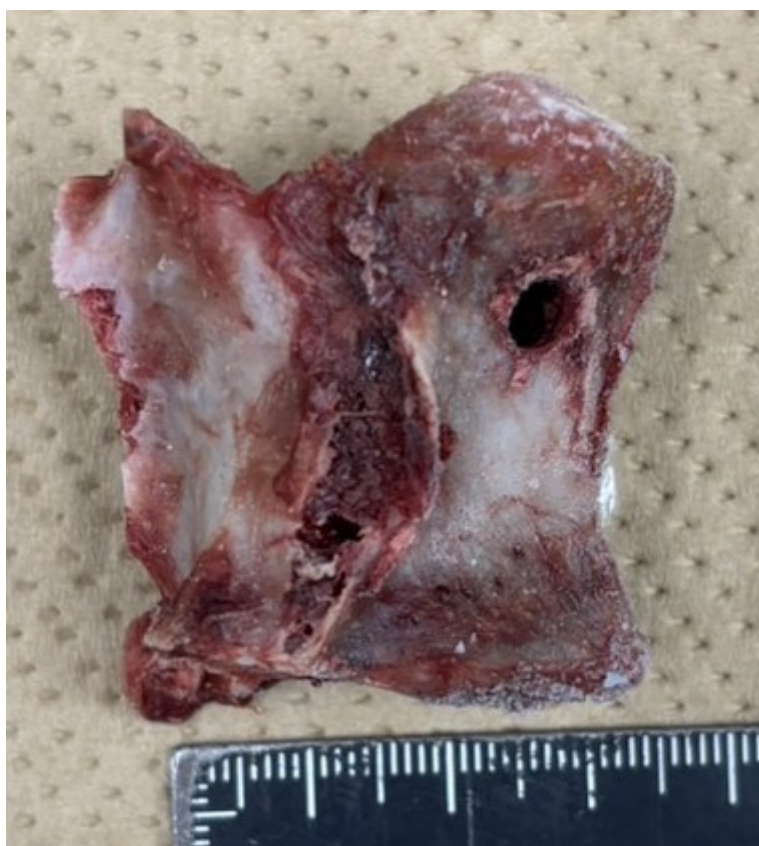
Fig. 4.2 Test specimen after drilling a prepared hole in the lumbar spine
