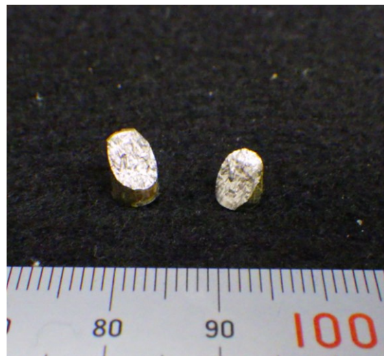
Fig. 4-3 The specimens of \text{Zr}_{55}\text{Cu}_{30}\text{Al}_{10}\text{Ni}_5 bulk metallic glass after compressive test ; (a) plastic deformation under low stress and (b) brittle fracture under high stress.
