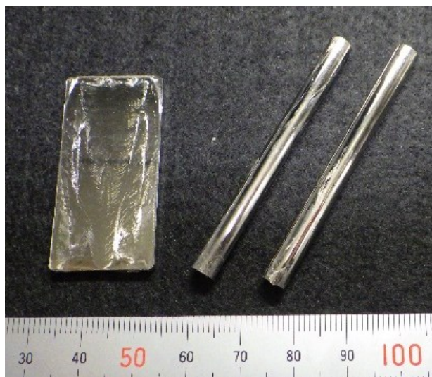
Fig. 3-1 Plate and round bar of \text{Zr}_{55}\text{Al}_{10}\text{Cu}_{30}\text{Ni}_5 bulk metallic glass produced by Orbray Corporation.
