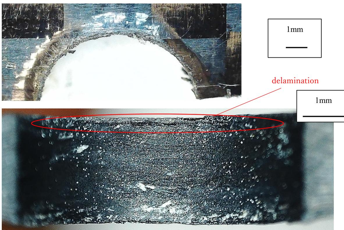
Fig.20 Processed hole with delamination at the edge.
