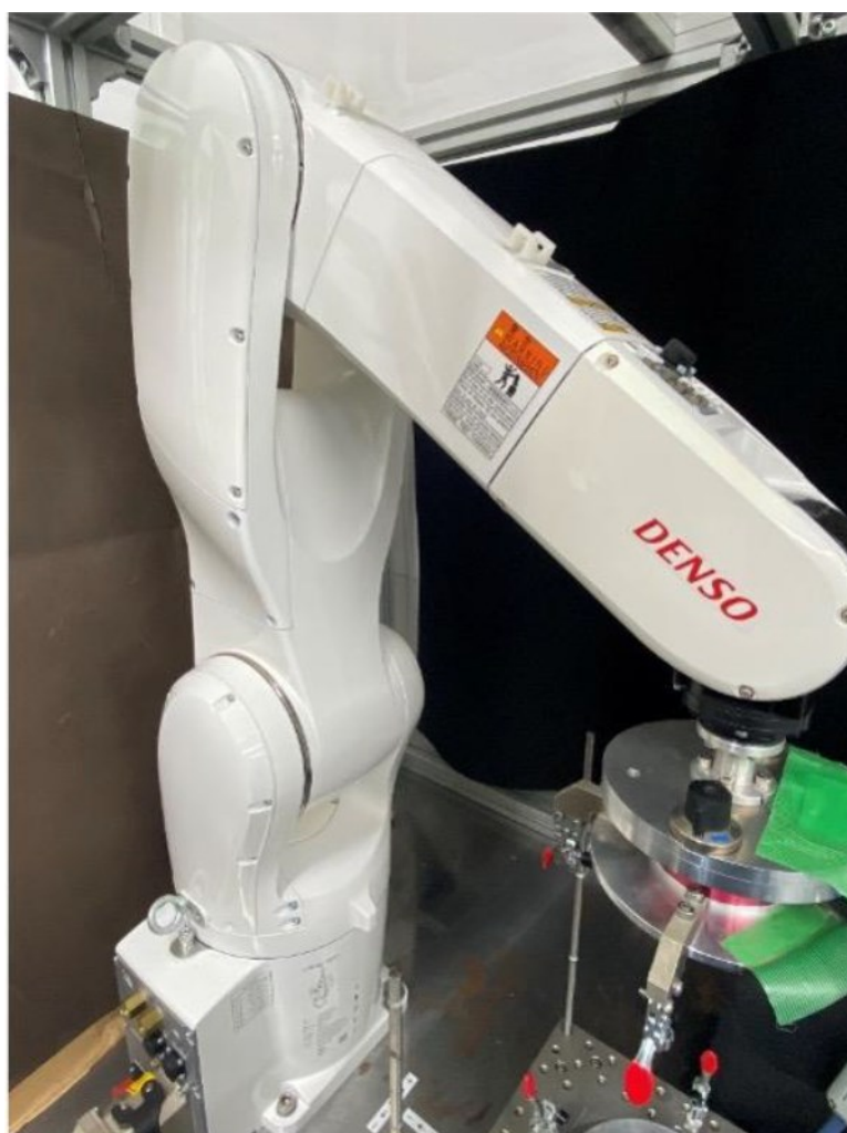
Fig. 4.13 6-axis testing machine with a serial mechanism
