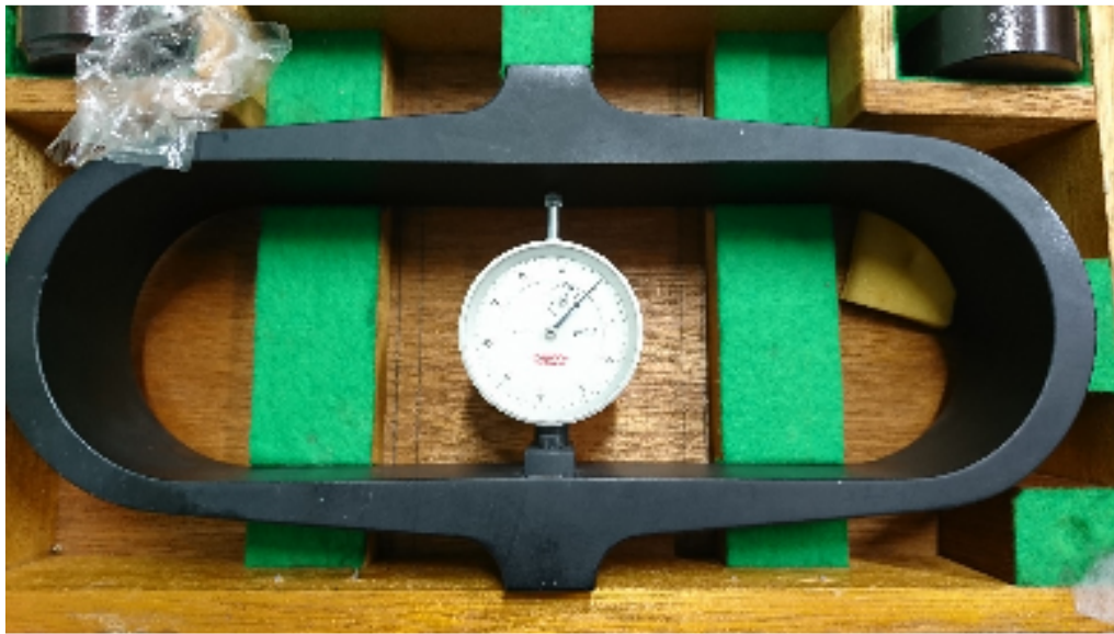
Fig.2.22 環状ばね型力計の外観
