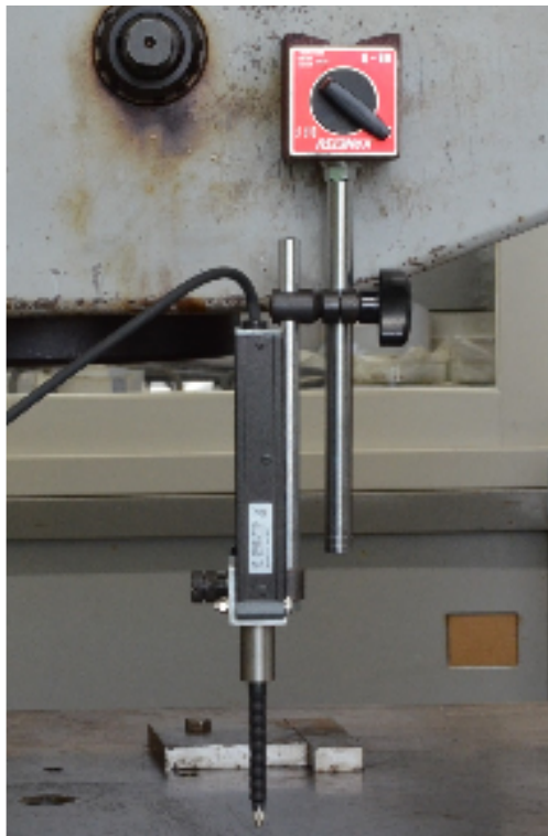
Fig.2.20 変位測定機 (ONO SOKKI 製 LINEAR GAUGE SENSOR GS-3830B)
