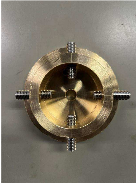
Fig.3.8 Specimen fixing jig
