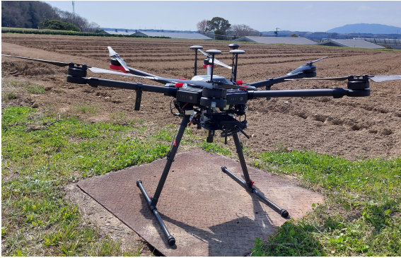
Figure 5.2: DJI M600 pro drone with the camera mounted
